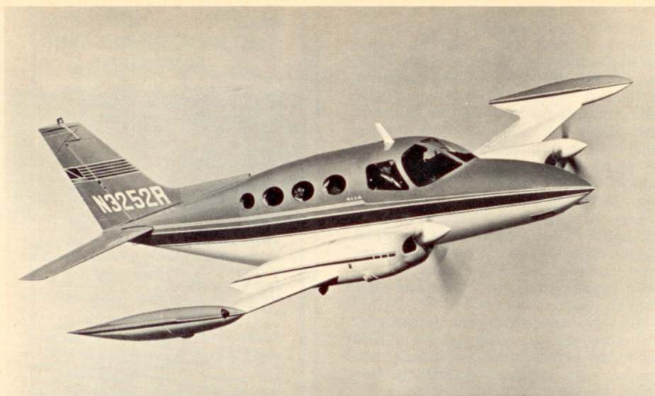
Cessna's "top of the line" Model 411-A reportedly offers many improvements for 1967, particularly in baggage-carrying capability and passenger comfort. The six-to eight-place executive twin will cruise over 1,100 miles at 246 m.p.h. in standard configuration at 20,000 feet, Cessna officials claim.
